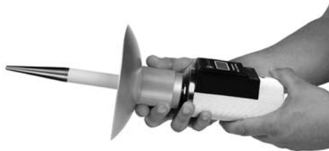
Figure B. Screw sensor to tester body
